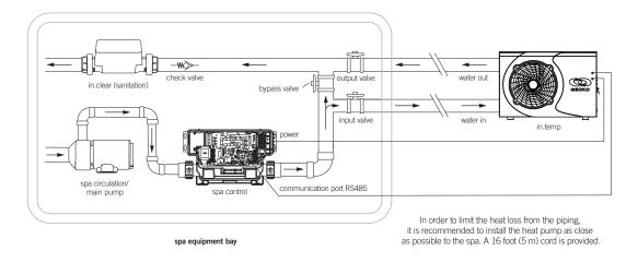
If your installation is equipped with a water treatment system (chlorine, bromine, salt, etc.) the bypass must be installed before the water treatment, with a check valve between the bypass and water treatment system.
